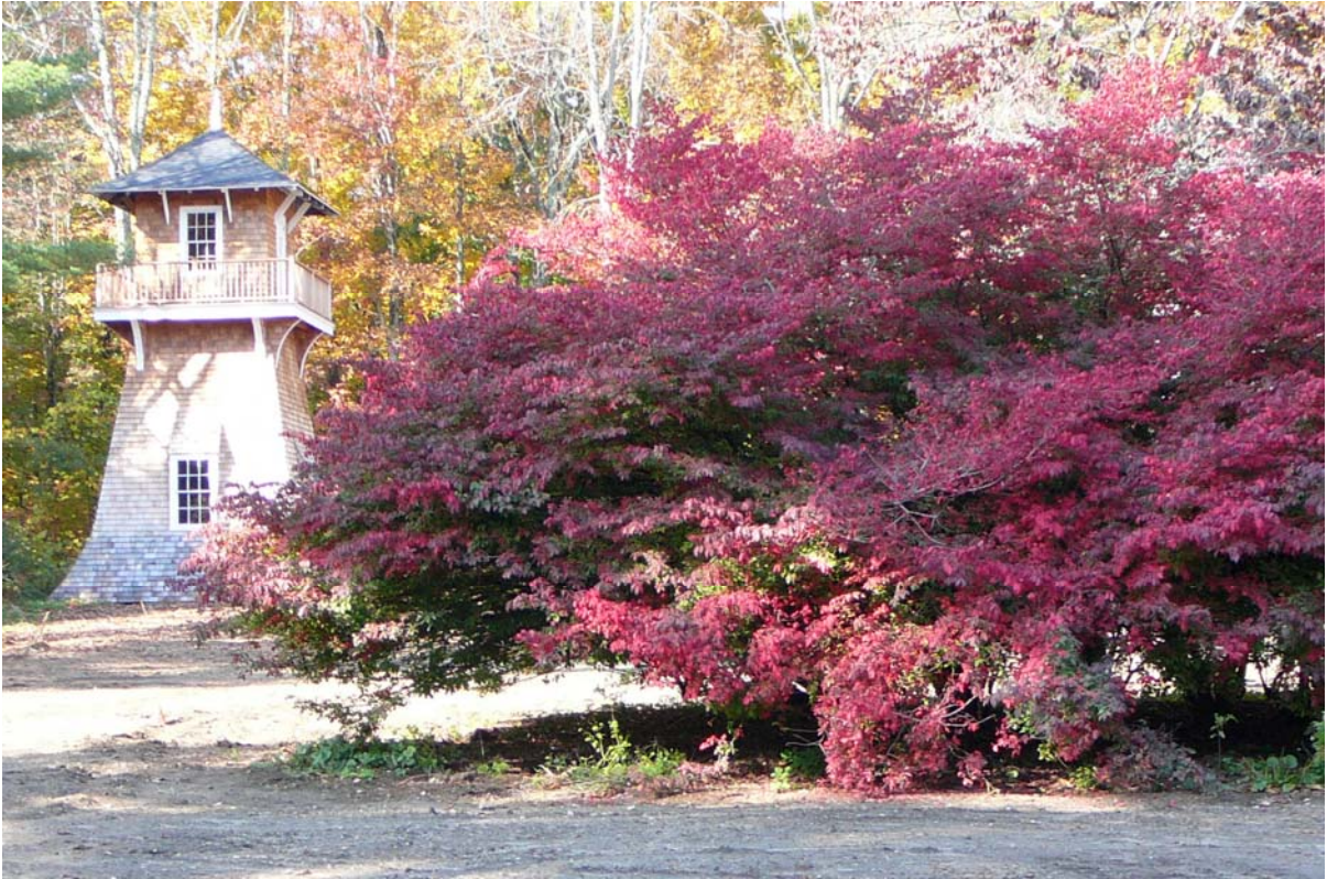
The John Otis water tower built in the late nineteenth century is one of several water towers located in the Town of Norwell. The purpose of the tower was to provide an attractive enclosure around a storage tank supported thirty feet above ground which supplies water on an as-needed basis by a gravity system, distributing water around the property.
