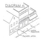
**Projection:** An extension forward or out from a wall of a building.
